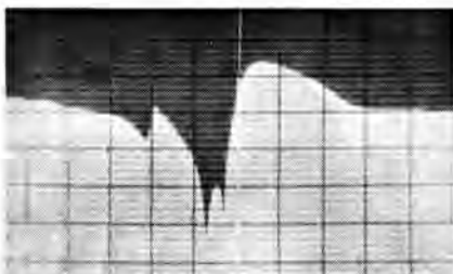
Response to prototype filter, horizontal scale 10MHz/div., vertical scale 10dB/div., bright line at 100MHz
